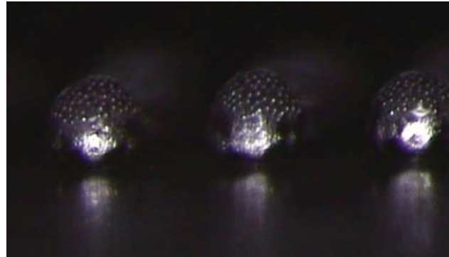
Figure 7-2 BGA Balls After Paste Dipping (Figure source: Indium Corporation)
