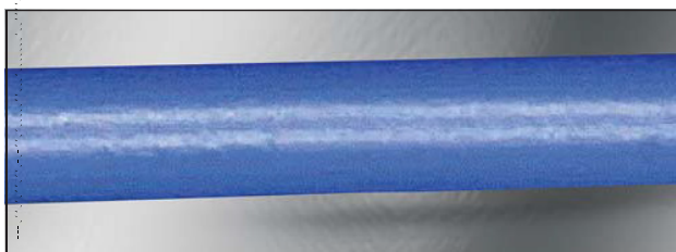
Figure 8-80 Example of Undamaged Insulation Jacket
