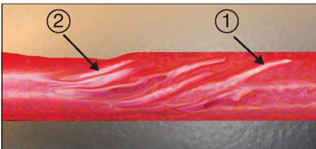
Figure 8-83 Creasing/Rippling of Outer Jacket 1. A1A2A3: Crease/ripple does not exceed insulation jacket thickness. 2. D1D2D3: Crease/ripple exceeds insulation jacket thickness.
