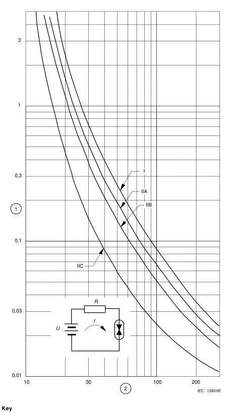
1 Minimum ignition current *I* (A) 2 Source voltage *U* (V)
